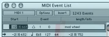
Figure 3-17: The Controller Event entry window has fields for the start time, controller number, and value.
